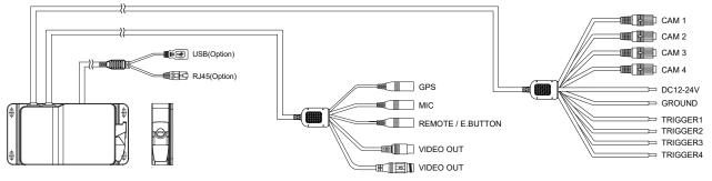
\* The two VIDEO OUT cables are configured with the same specification (HD, FHD, or CVBS) as preset at the time of shipment.
